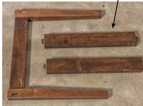
leg assembly glued & pocket-screwed
